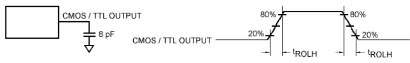
FIGURE 5. Receiver LVTTTL/CMOS Output Load and Transition Times
